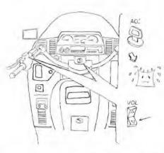
When the ignition switch is turned OFF, the AM/FM radio preset memory and clock will continue to function with the back-up power supply circuit from the battery. But resetting is required when the battery becomes totally discharged or is disconnected.
